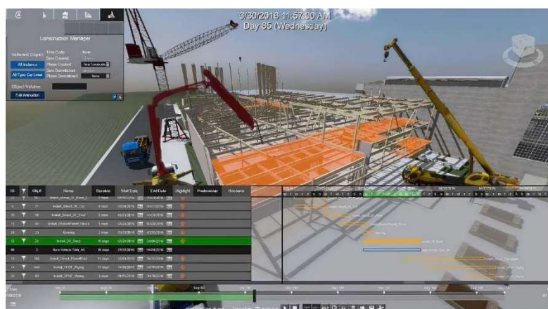
Figure 4. BIM-based construction simulation of prefabricated utility tunnels
