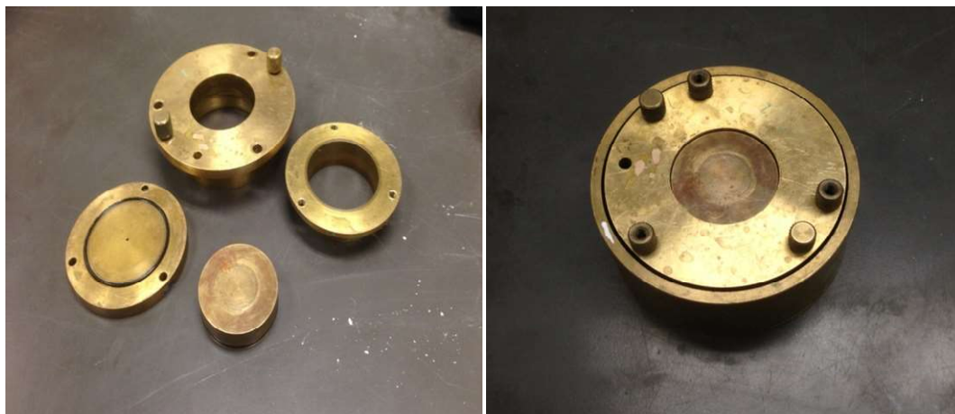
Fig. 9 Special designed oedometer cell (the diameter of the ring is 50.80mm).
