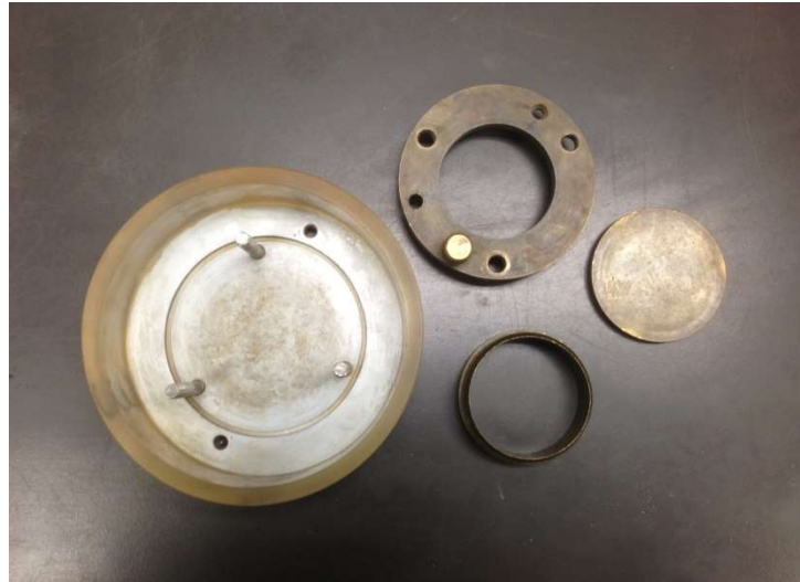
Fig. 10 Oedometer cell for Bishop type oedometer (the diameter of the ring is 50mm).
