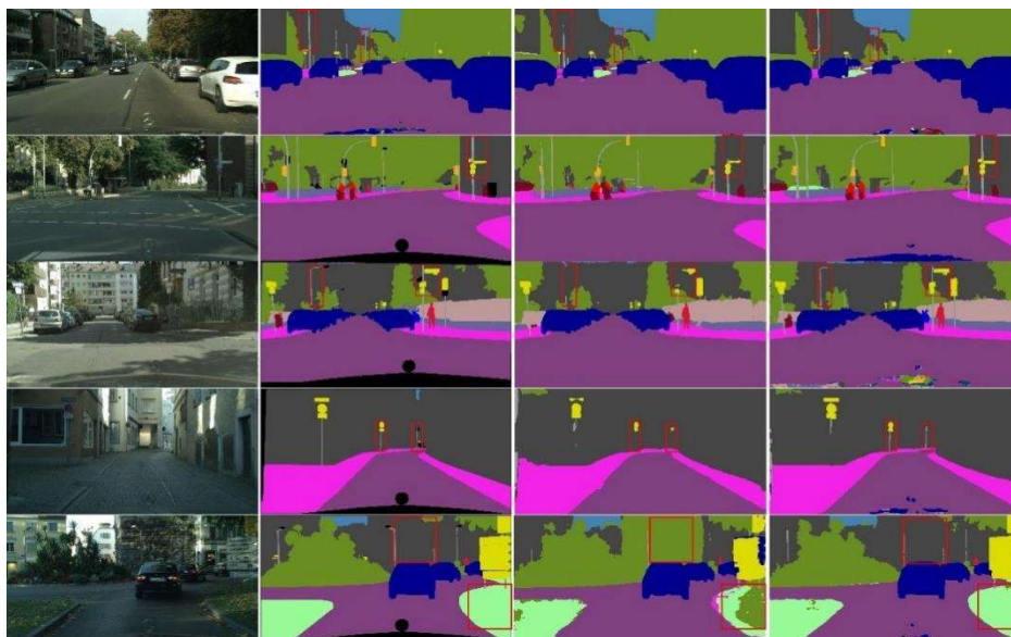
Figure 5. Comparison of segmentation results. (a), (b), (c) and (d) represent original images, labeled images, the results of PP-LiteSeg and those of MFF-LiteSeg, respectively.
