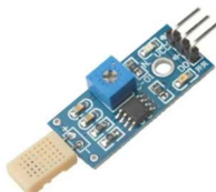
Figure 4. Humidity detection module
