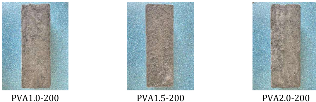
Figure 3. PVA-ECC freeze-thaw appearance damage example diagram
