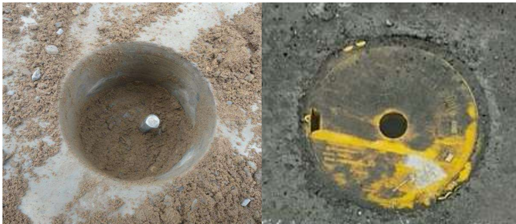
Figure 3. Photos of Ground Surface Settlement Monitoring Points
