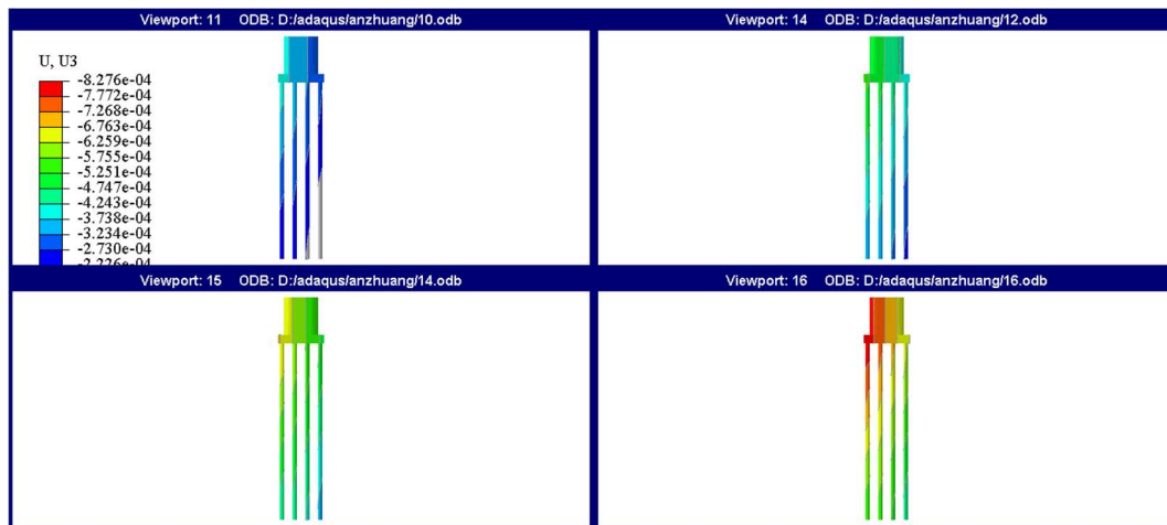
Figure 15. Bridge Pile Settlement under Different Dewatering Durations
