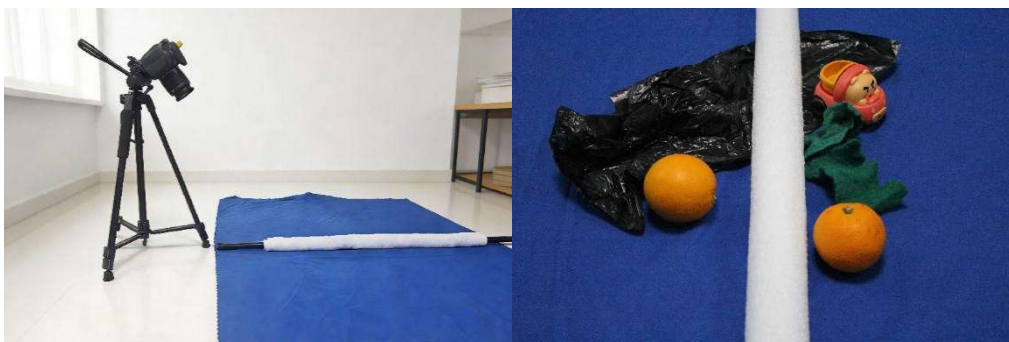
Figure 10. Indoor simulated ice-coated conductor shooting scene and original shooting images
