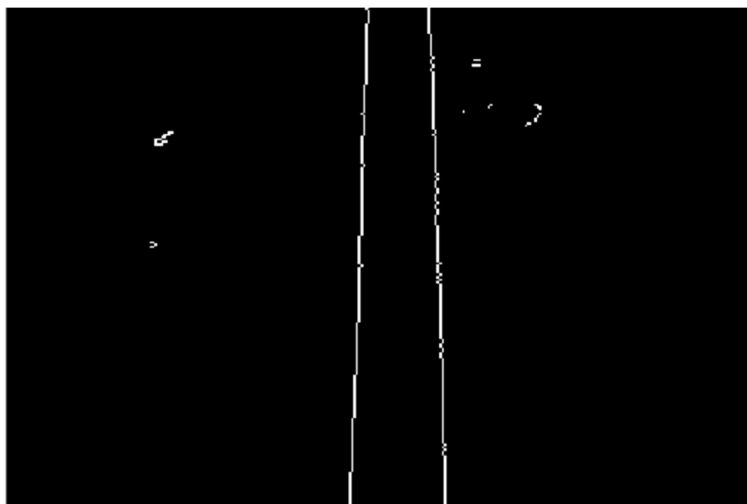
Figure 12. Detection result of indoor simulated ice-covered conductor using the improved Canny operator
