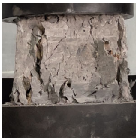
Figure 4. Failure process of carbon fiber concrete
