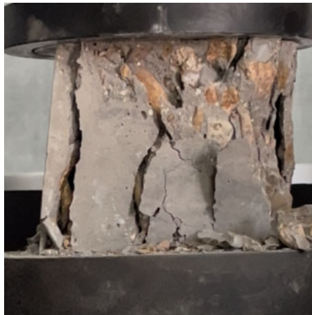
Figure 3. Failure process of ordinary concrete
